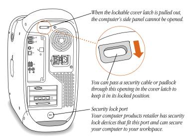
Follow the instructions supplied with the locking cable to secure it to your computer. When you install the locking cable, feed the cable through the lockable latch on the cover to prevent memory, disk drives, and expansion cards from being removed.
