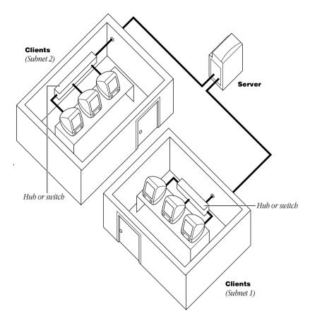
If this is your configuration, select Gateway in the IP Routing Configuration panel of the NetBoot Server Setup Assistant. You don't need to provide a router IP address.
