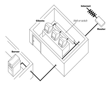
The server is a peer of NetBoot clients on a single subnet—each is connected directly to the router. If this is your configuration, select Peer in the IP Routing Configuration panel of the NetBoot Server Setup Assistant. For "Router IP address" enter the IP address of the router.
