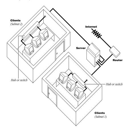
In this configuration, the server acts as a router to one or more NetBoot client subnets. If this is your configuration, select Gateway in the IP Routing Configuration panel of the NetBoot Server Setup Assistant. You do not need to provide a router address.
