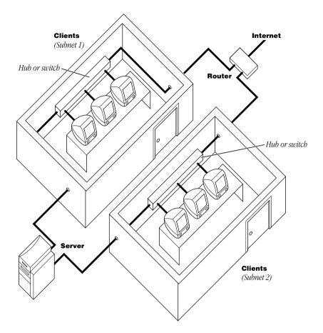
This configuration is similar to the previous one, except there are two NetBoot client subnets. Each subnet is connected to a different port on the router and a different port on the server. If this is your configuration, select Peer in the IP Routing Configuration panel of the NetBoot Server Setup Assistant. For "Router IP address" enter the IP address for the router port you connect to that subnet.
